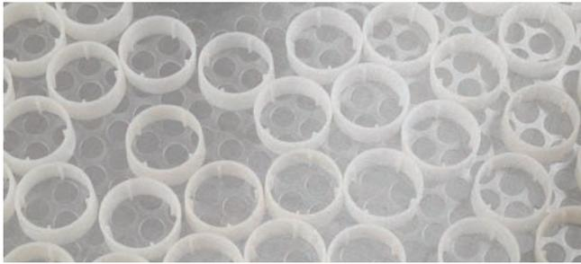
**Antiblinding devices, like the sliders shown here, help prevent particles from sticking in the screen openings.**
